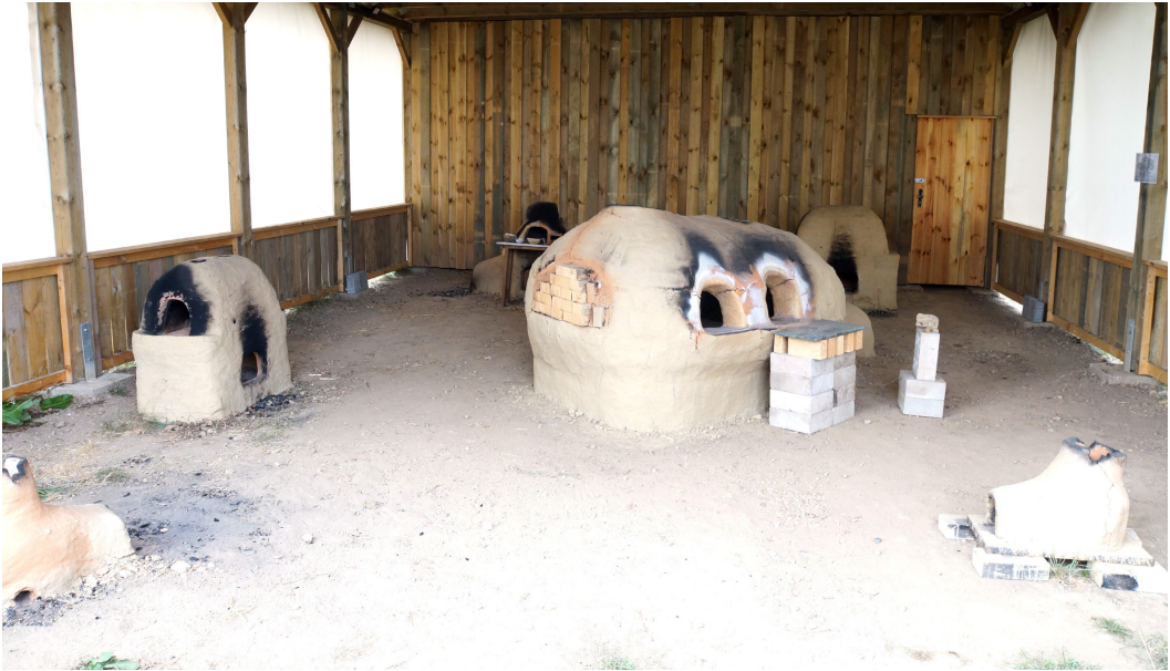
Abb. 3: Die neue Glashütte: Perlenofen PO-Borg-5, Kühlöfen KO-Borg-4, Schmelz-/Arbeitsöfen (Hafenöfen) GO-Borg-4, Wannöfen GO-Borg-3, Kühlöfen KO-Borg-3 und Perlenöfen KO-Borg-7 (von links nach rechts). – The new glass workshop: bead furnace PO-Borg-5, annealing oven KO-Borg-4, glass furnace (pot furnace) GO-Borg-4, tank furnace GO-Borg-3, annealing oven KO-Borg-3, and bead furnace KO-Borg-7 (starting from left).
