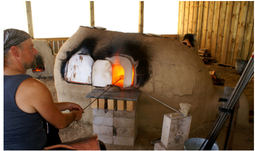
Abb. 5: Glas blasen direkt am Wannnofen GO-Borg-3. – Blowing glass directly in front of the tank furnace GO-Borg-3.
