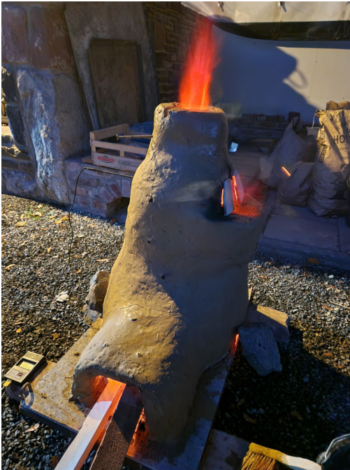
Abb. 3: Trockenbrennen des neuen Glasofens. – Dry firing the new glass furnace.
